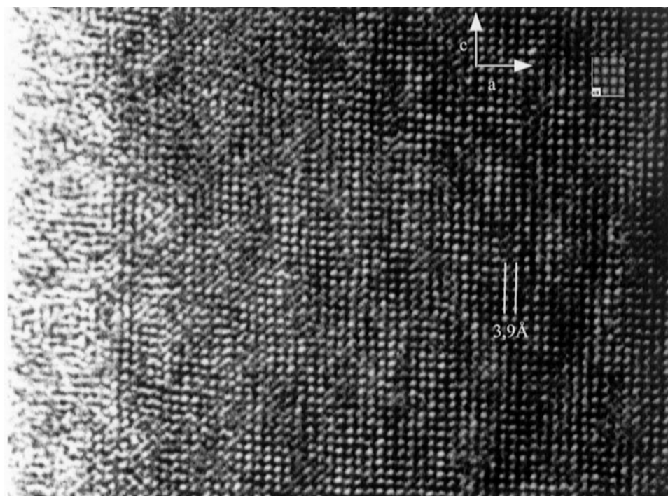
FIG. 10. HREM image of the orthorhombic mixed oxide V_{0.13}Mo_{0.87}O_{2.935} along [010].
